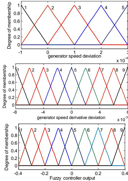
Fig. 6. Membership functions of inputs and output.
