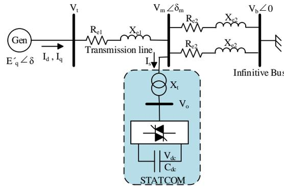
Fig. 1. SMIB system model with a STATCOM.
