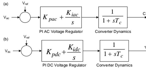
Fig. 2. STATCOM PI controller for (a) ac voltage and (b) dc voltage.
