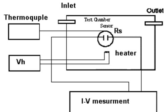
**Fig. 2.** Schematic diagram for AlGaN gas sensors measurement.  $V_H$ : heater voltage;  $R_S$ : AlGaN resistance.
