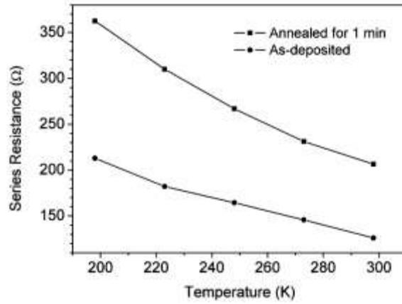
**Figure 5:** Temperature dependence of series resistance of the Schottky contacts without annealing and annealed in 2% hydrogen in nitrogen ambient for 1 min.
