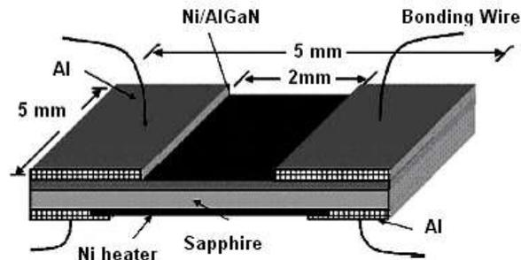
**Fig. 1.** Structure of a Ni/ AlGaN gas sensor.
