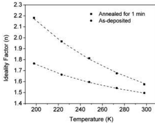
**Figure 4:** Temperature dependence of the ideality factor of the Schottky contacts without annealing and annealed in 2% hydrogen in nitrogen ambient for 1 min. The dashed curves represent the theoretical temperature dependence of the ideality factor.
