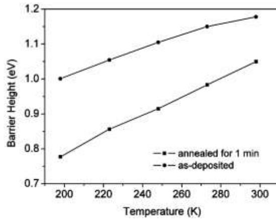
**Figure 6 :** Temperature dependence of the barrier height of the Schottky contacts without annealing and annealed in 2% hydrogen in nitrogen ambient for 1 min.
