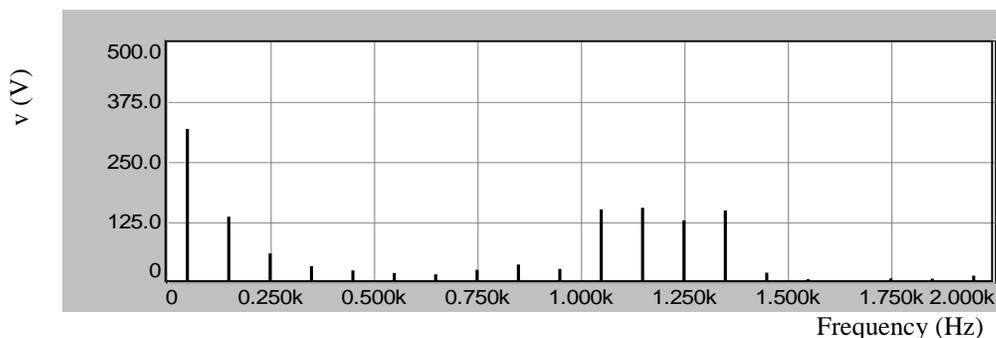
(b) Harmonic spectrum of voltage waveform presented in Fig. 5
