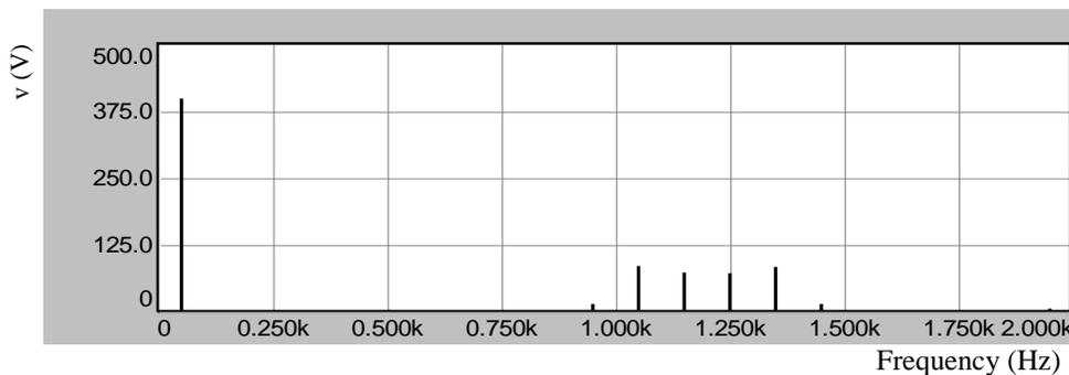
(a) Harmonic spectrum of voltage waveform presented in Fig. 7
