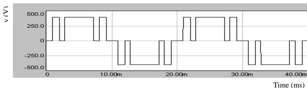
(a)  $f_o = f_r = 50$  Hz,  $f_c = 400$ Hz
