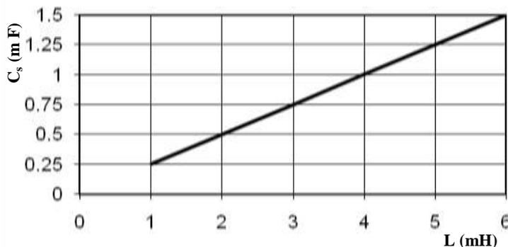
Fig. 6 Relation between load inductance ( $L$ ) and snubber capacitance ( $C_s$ )
