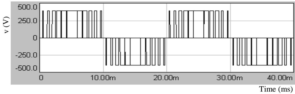
Fig. 8 Output voltage waveform of the PWM inverter feeding an inductive load
