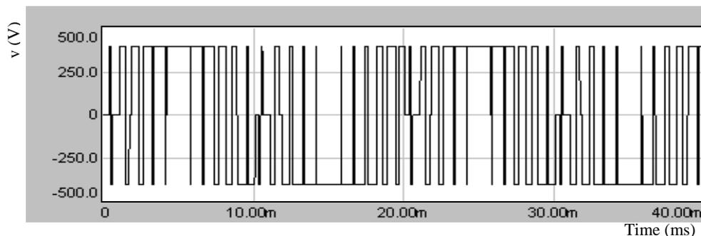
Fig. 5 Output voltage waveform of the PWM inverter feeding an inductive load (without snubber circuit)
