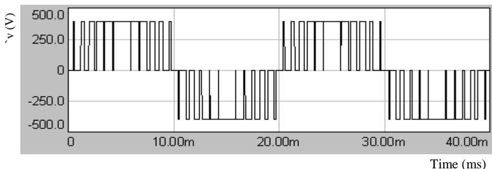
Fig. 7 Output voltage waveform of the PWM inverter feeding an inductive load (R = 2 Ohm and L = 5 mH, R<sub>s</sub> = 2 Ohm, C<sub>s</sub> = 1.25 mF)
