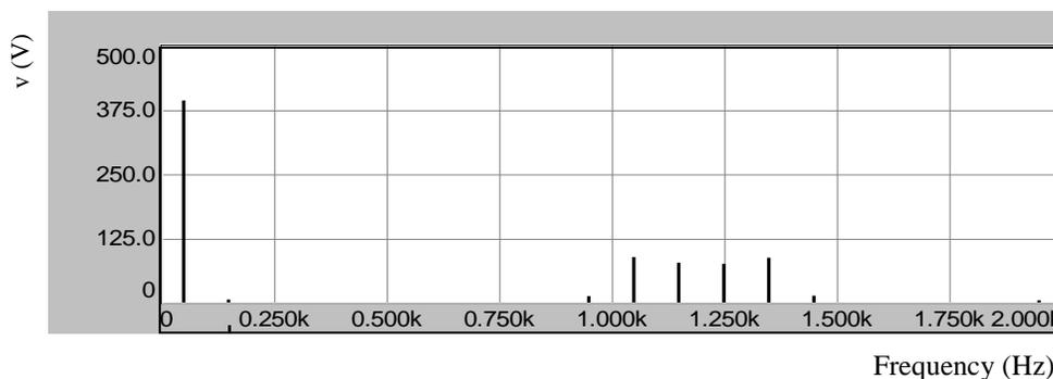
(c) Harmonic spectrum of voltage waveform presented in Fig. 9 (a)
