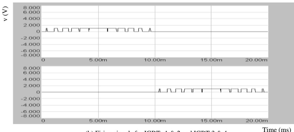
(b) Firing signals for IGBTs 1 & 2 and IGBT 3 & 4
