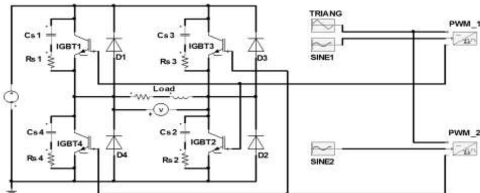
Fig. 1 Power and control circuit of a 1- $\phi$  PWM inverter
