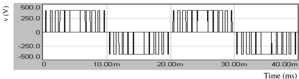
(b)  $f_o = f_r = 50$  Hz,  $f_c = 1200$ Hz
