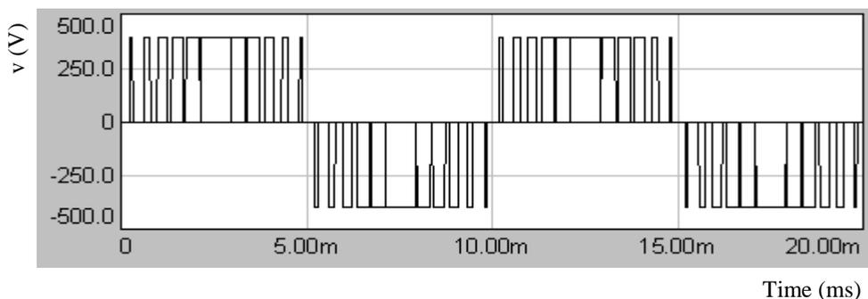
(a)  $f_o = 100$  Hz,  $f_c = 2400$  Hz,  $R = 2$  Ohm and  $L = 5$  mH,  $R_s = 2$  Ohm,  $C_s = 1.25$  mF
