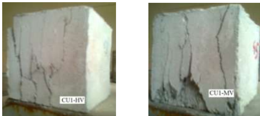
Fig. 6 Sample of cube specimens after failure
