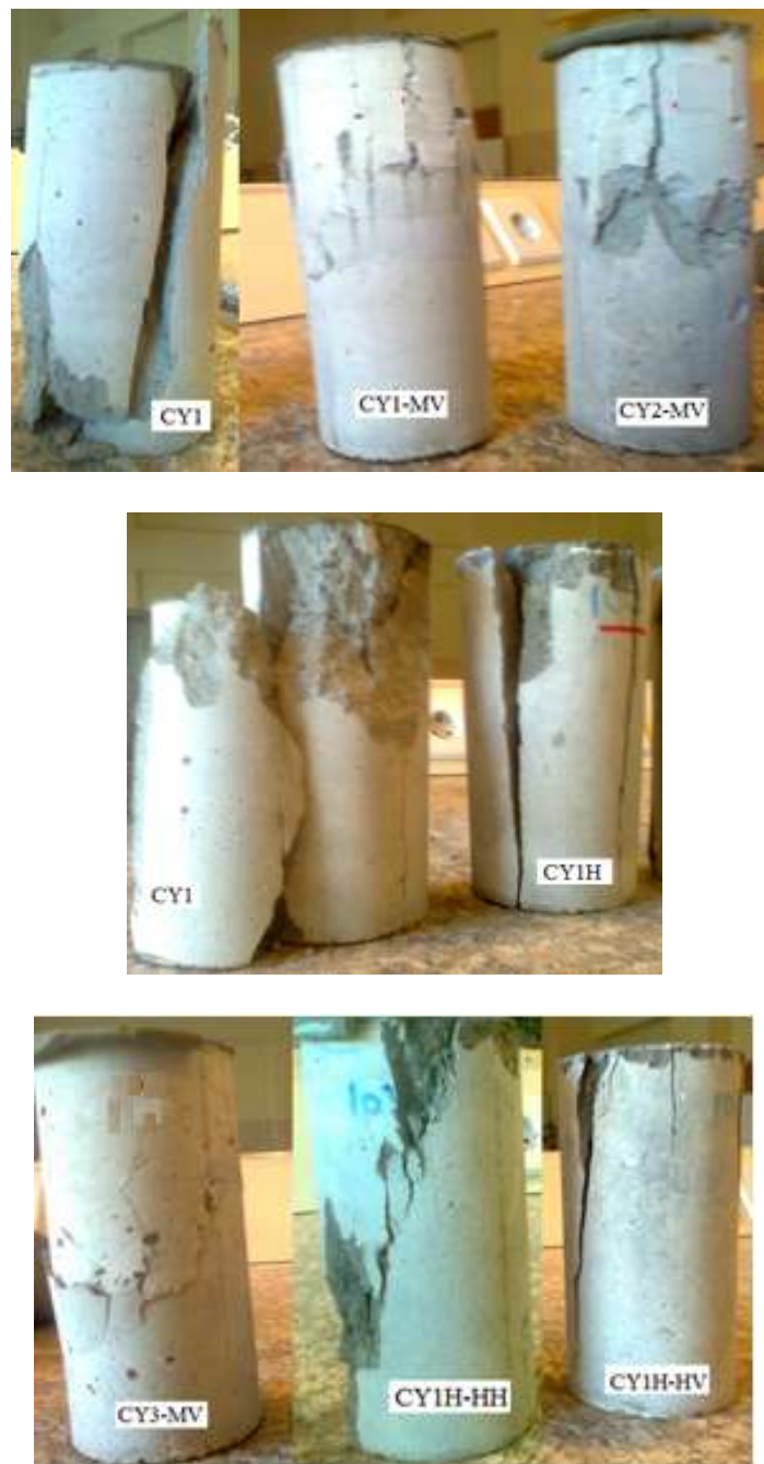
Fig. 7 Sample of cylinder specimens after failure
