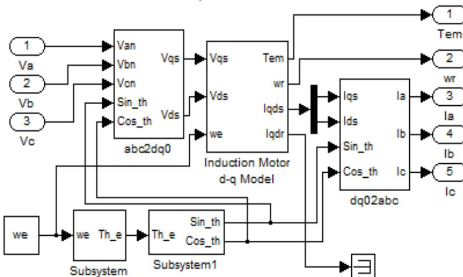
Fig. 2. matlab simulink model of proposed system
