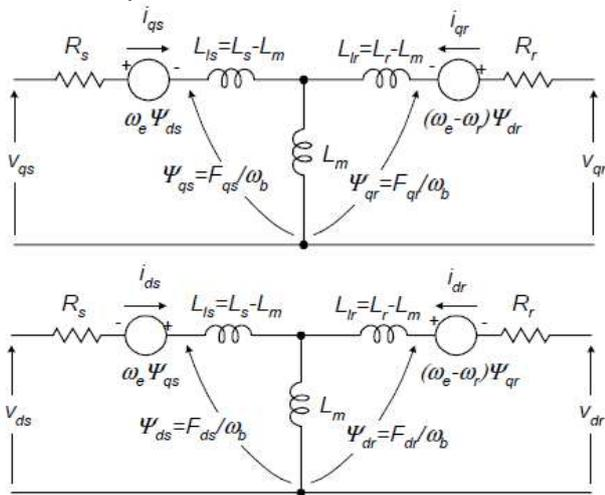
Fig. 1. Dynamic or d-q equivalent circuit of an IM
