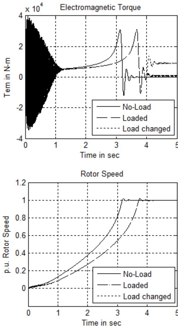
Fig. 5. Electromagnetic torque and p.u. Rotor speed for M3
