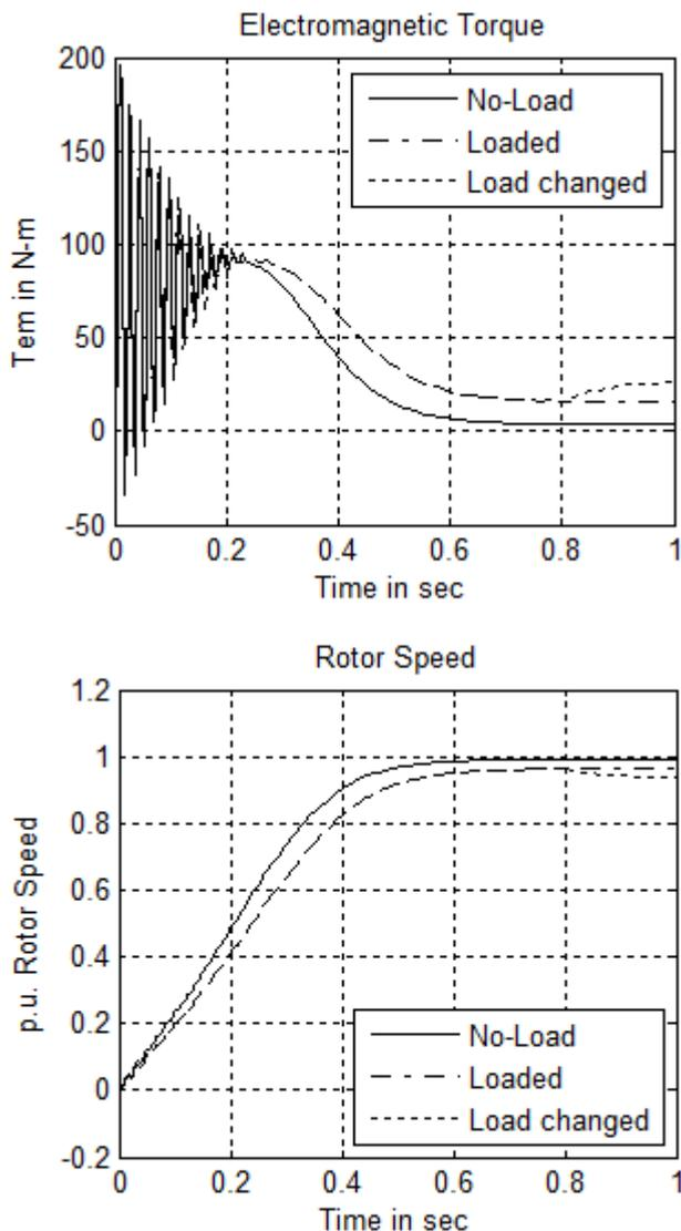
Fig. 3. Electromagnetic torque and p.u. Rotor speed for M1.
