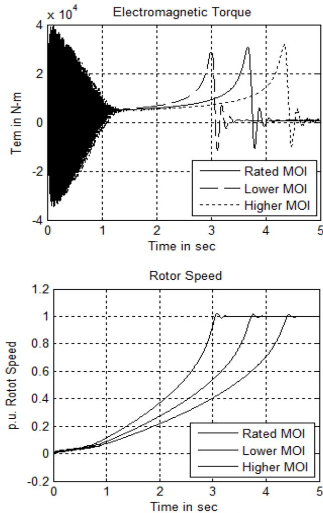
Fig. 8. Electromagnetic torque and p.u. Rotor speed for M3.
