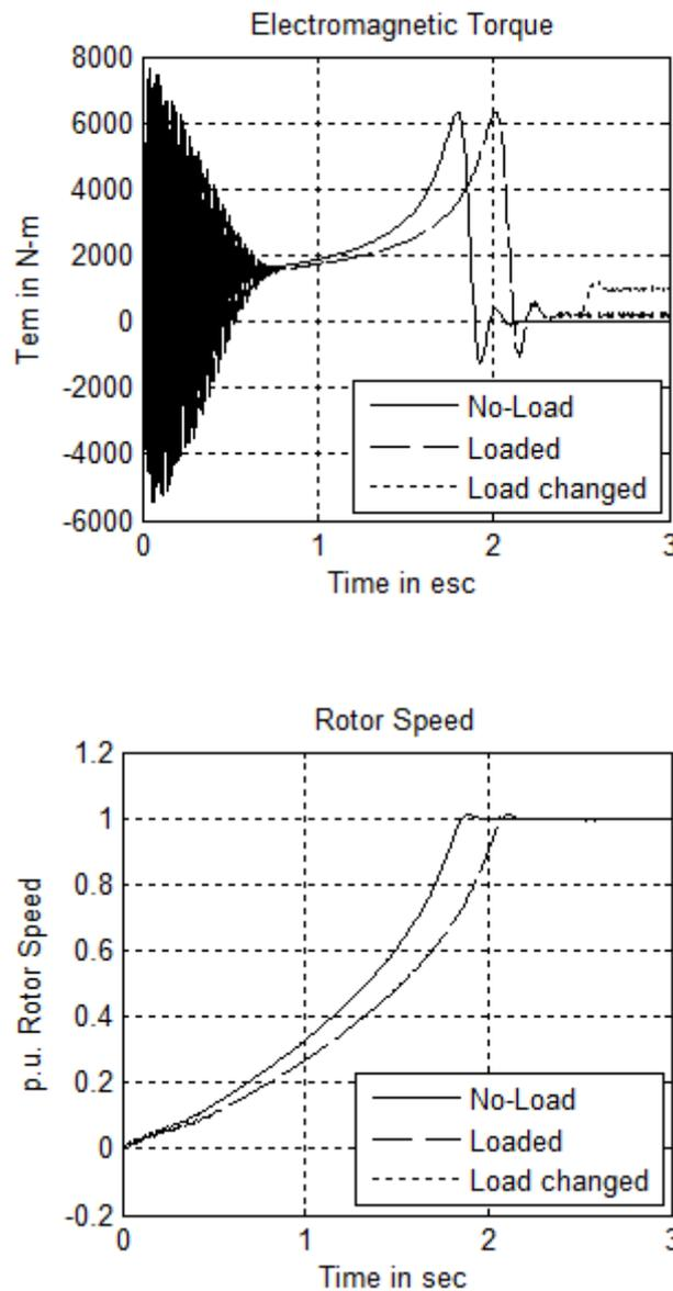
Fig. 4. Electromagnetic torque and p.u. Rotor speed for M2.
