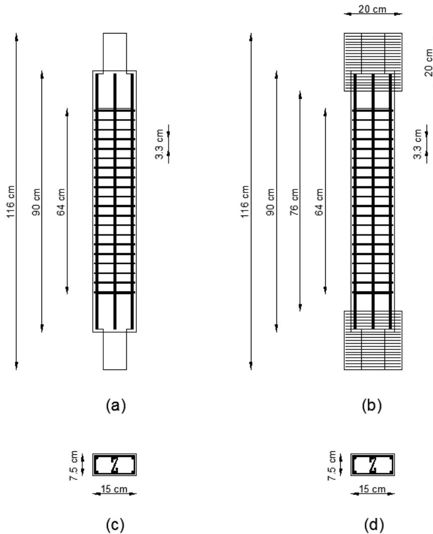
Fig. 2. Column specimen Y-6Ø8-268-30-1: (a) Front view in tension, (b) Front view
