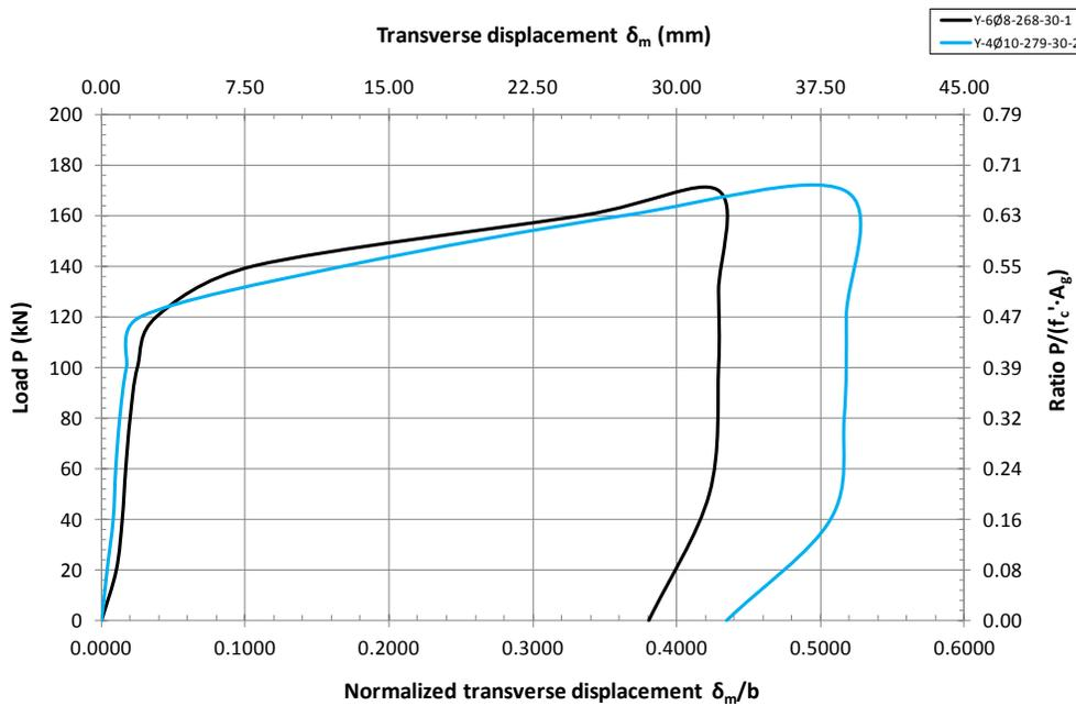
Fig. 5. Diagram of compressive load [P(kN), P/(f<sub>c</sub>'·A<sub>g</sub>)] - transverse displacement at the midheight of test specimens [ $\delta_m/b$ ,  $\delta_m(\text{mm})$ ].
