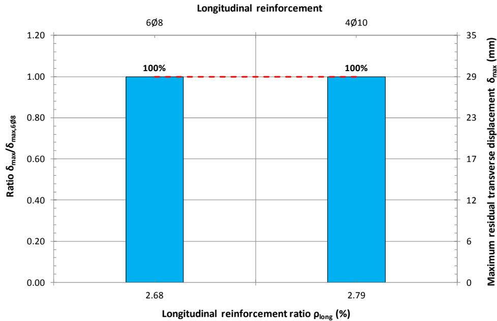
Fig. 9. Column diagram of maximum residual transverse displacement [ $\delta_{max}/\delta_{max,1.79\%}, \delta_{max}(mm)$ ] – longitudinal reinforcement ratio and type of longitudinal reinforcement [ $\rho_{long}(\%)$ ].
