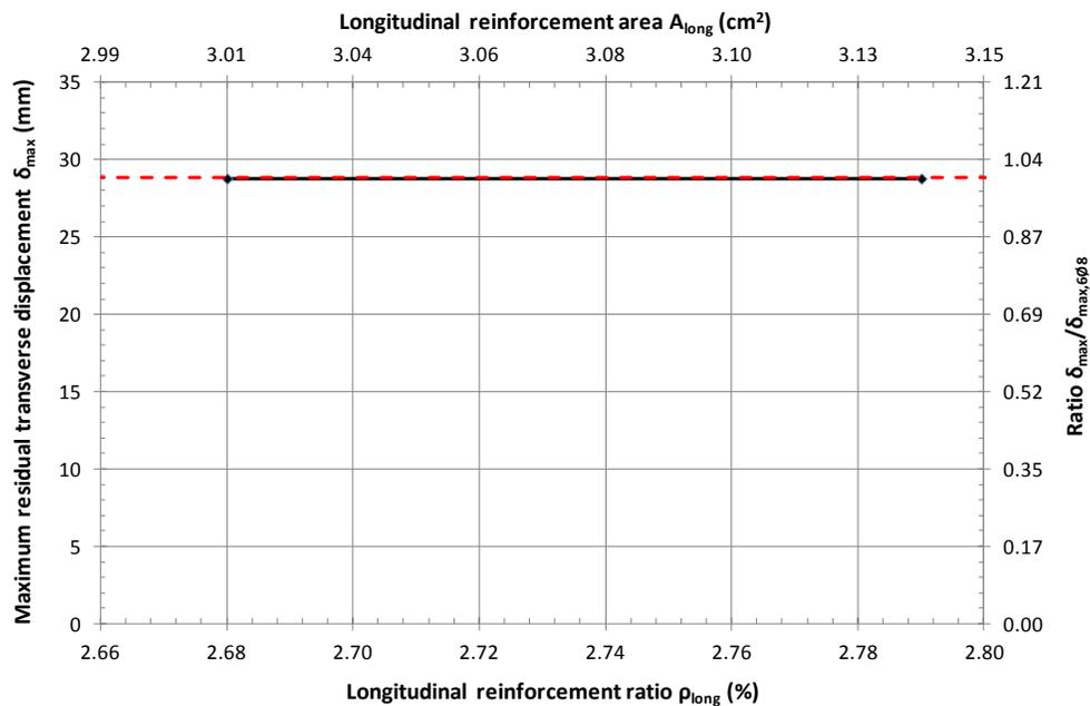
Fig. 8. Diagram of maximum residual transverse displacement [ $\delta_{max}$ (mm),  $\delta_{max}/\delta_{max, 1.79\%}$ ] – longitudinal reinforcement ratio and longitudinal reinforcement area [ $\rho_{long}$ (%),  $A_{long}$ (cm<sup>2</sup>)].
