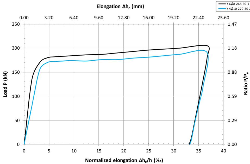
Fig. 4. Diagram of tensile load [P(kN), P/P<sub>y</sub>] - elongation [ $\Delta h_e/h(\%)$ ,  $\Delta h_e(\text{mm})$ ].
