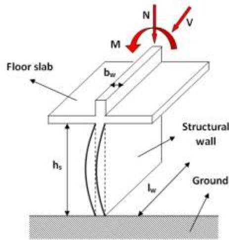
Fig. 1. Out-of-plane buckling of structural wall.
