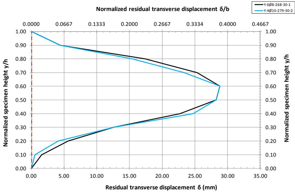
Fig. 6. Diagram of normalized specimen height  $[z/h]$  – residual transverse displacement  $[\delta(\text{mm}), \delta/b]$ .
