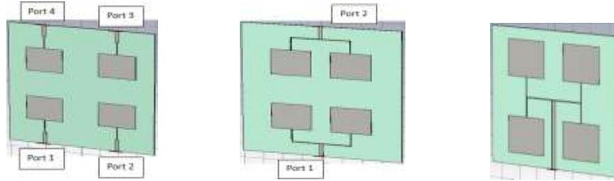
Fig. 5. The Square Array with (a) Four Individual Feeds (b) Two feeds (c) Single Feed
