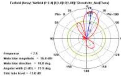
Fig. 19. The Beam Pattern for 0,90 ( $\alpha=90$ ) for Linear Two Feeds Array
