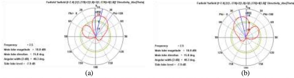
Fig. 23. The Beam Pattern for (a) 270,0,-270,0 and (b) -270, 0, 270, 0 for Square Array with four Feeds
