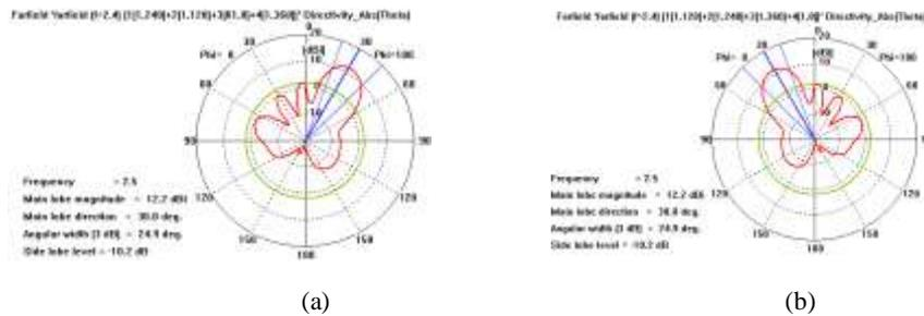
Fig. 14. The Beam Patterns for (a) 0,120,240,360 and (b) 360,240,120,0 for Linear Individual Feed Array
