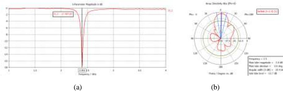
Fig. 20. (a) S-Parameter and (b) Beam Pattern for Linear Array with Single Feed
