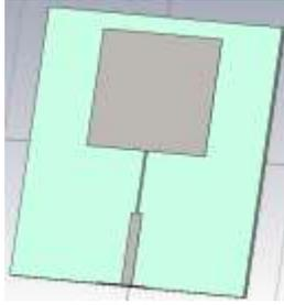
Fig. 2. Single patch Micro strip antenna
