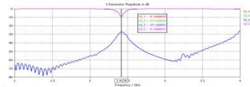
Fig. 15. The S-Parameter for Linear Array with Two feeds
