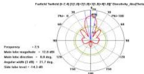
Fig. 10. The Beam Pattern for  $\alpha=0$  for Linear Individual Feed Array
