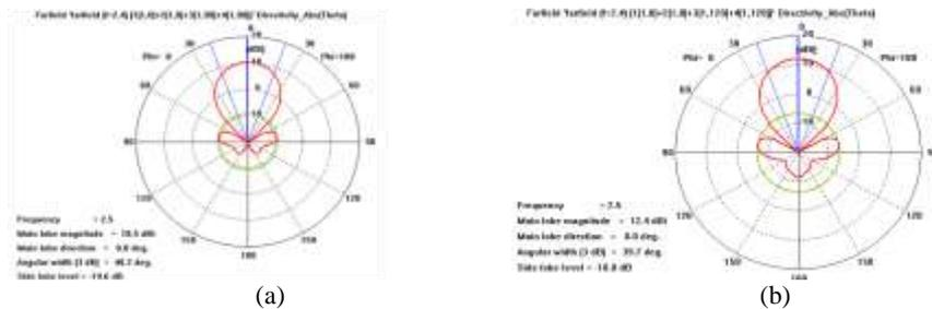
Fig. 22. The Beam Pattern for (a) 0,0,90,90 and (b) 0,0,120,120 for Square Array with four Feeds
