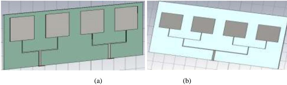
Fig. 4. The Linear Array with (a) Two Feeds and (b) Single Feed
