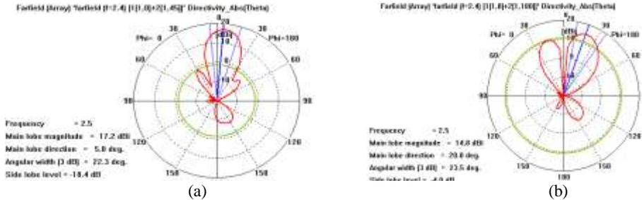
Fig. 17. The Beam Patterns for (a) 0,45 ( $\alpha=45$ ) and (b) 0,180 ( $\alpha=180$ ) for Linear Two Feeds Array
