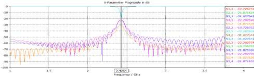
Fig. 21. The S-Parameters for Square Array with Four Feeds
