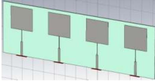
Fig. 3. Linear Array with Individual Feeds
