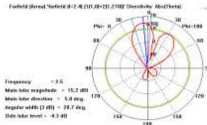
Fig. 18. The Beam Pattern for 0,270 ( $\alpha=270$ ) for Linear Two Feeds Array
