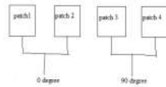
Fig. 7. The Equivalent Model with Two Feeds
