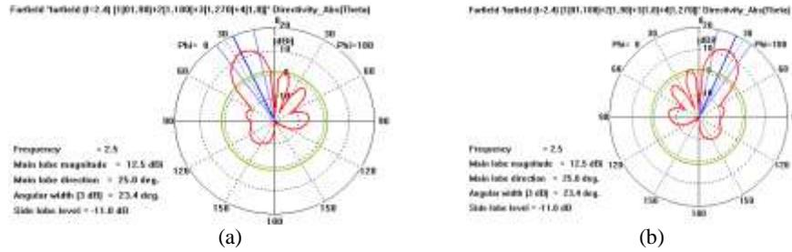
Fig. 13. The Beam Patterns for (a) 180,270,90,0 and (b) 0,90,270,180 for Linear Individual Feed Array
